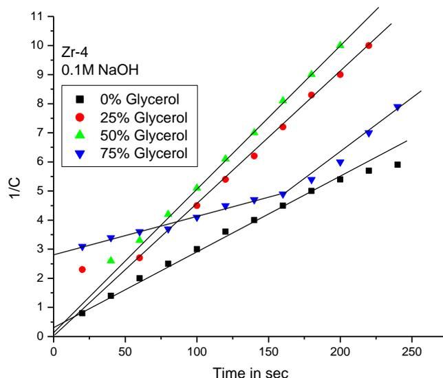
**TABLE-1: Effect of solvent on the anodization of zircaloy-4 in 0.1M sodium hydroxide.**
